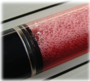
Demonstrate cavitation and pseudo-cavitation - Occurs when inlet is restricted or when there is an air leak present
